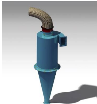
3D CAD modelling of Cyclone Separator
