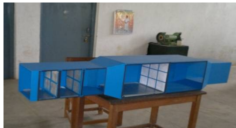
Fig. 7 filter unit with three stages of filters
